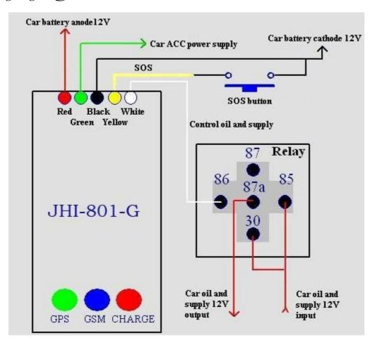
The external 5 wires of TLT-2H GPS/GSM tracker are as follows. Red for the 12V car power wire, connect to the car battery anode; Black for the earth GND, connect to the car battery cathode; Yellow for the SOS for help Control wire, connect external SOS switch button to car battery
